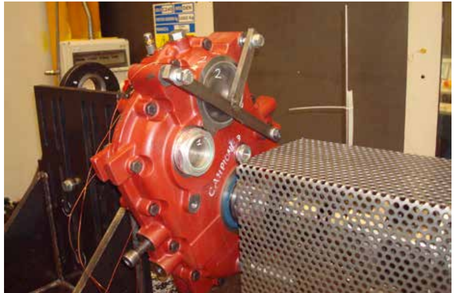
Fig. 4. At higher input speeds transfer box temperatures are superior to the ones at lower input speeds, due to the higher power losses, especially near bearings and seals.
