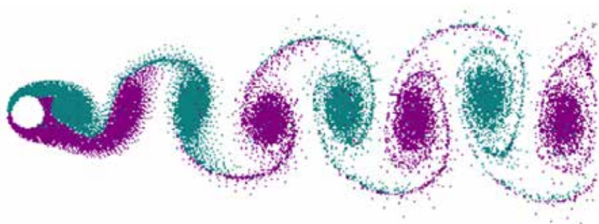
Fig. 11. Phenomenon of alternating vortex shedding. (credit: https://en.wikipedia.org/wiki/Vortex_shedding | Cesareo de La Rosa Siqueira)
