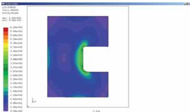
Fig. 4 - The CalculiX GraphiX window, where the von Mises stress for the C-shaped plate is plotted.
