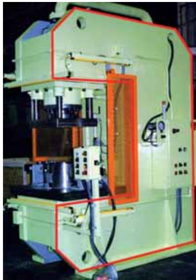
Fig. 1 - An example of C-type press. The steel C-shaped profile which will be optimized in this work is highlighted with a red line.
