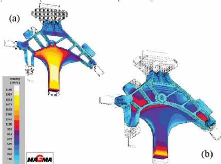
**Fig. 3:** Velocity field at 70% of filling: section (a) and overall view of the bracket (b).
