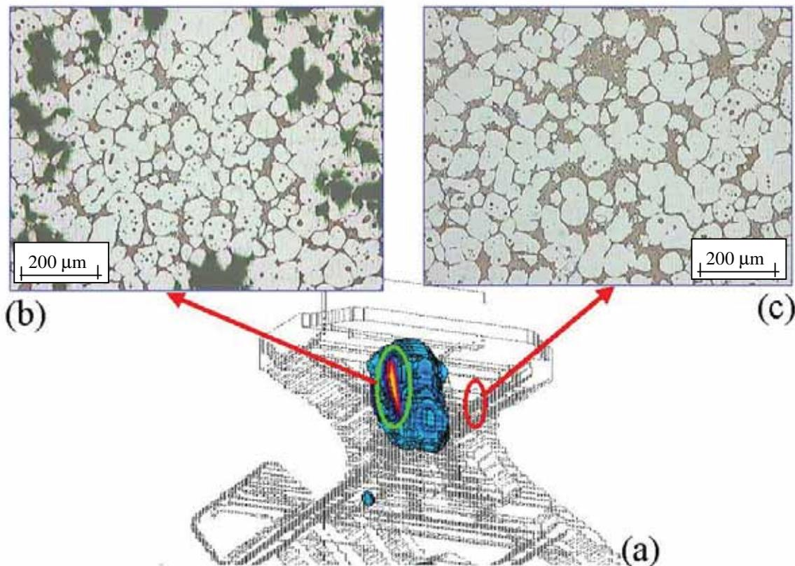
**Fig. 7:** Upper part of the casting: last region to solidify, as individuated by numerical simulation (a); corresponding microstructure with presence of microporosity (b), compared with that of a region with lower solidification times (c).
