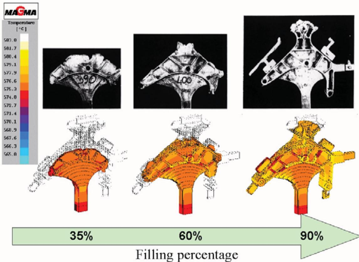
**Fig. 2:** Filling sequence: comparison between interrupted filling tests and numerical simulation results.
