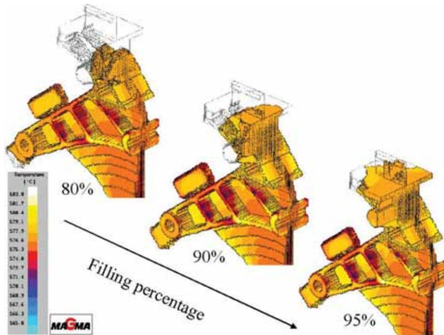
**Fig. 4:** Final part of filling sequence (upper region of the engine bracket).
