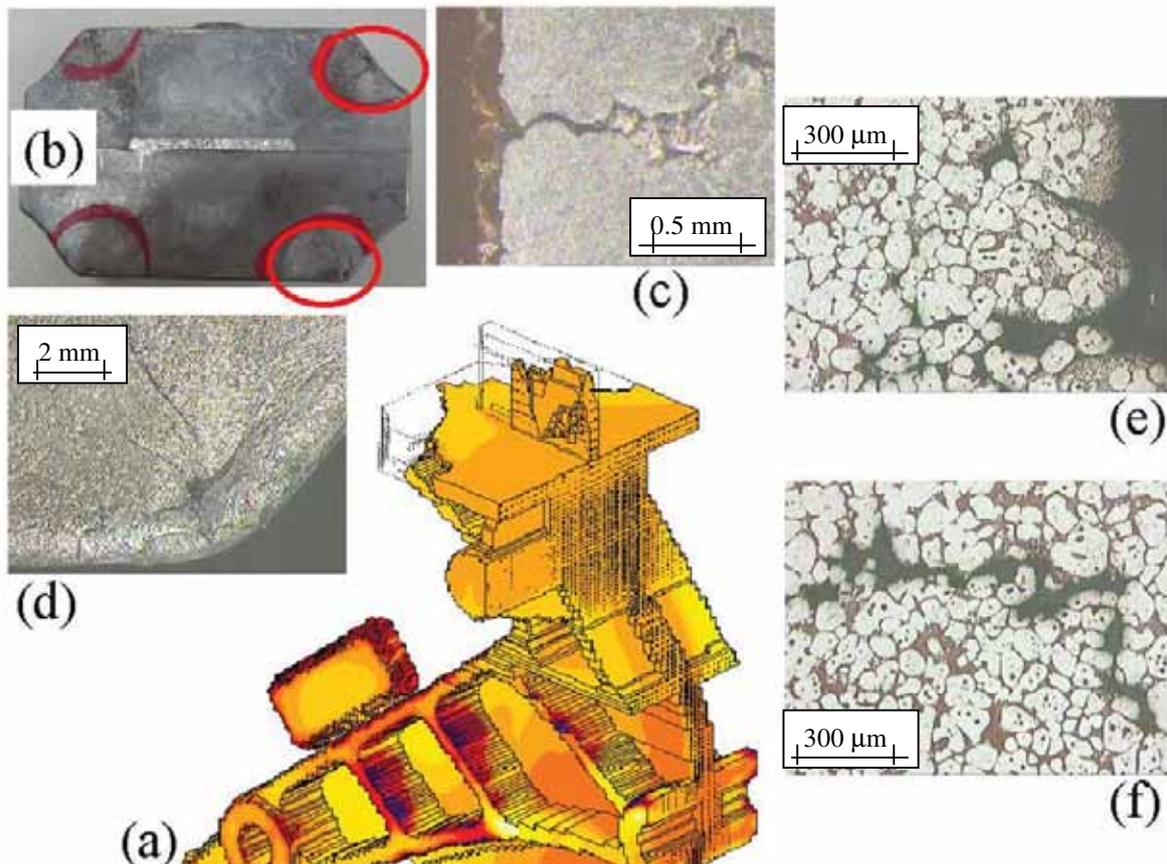
**Fig. 5:** Final stage of filling in the upper part of casting (a); photo of the upper plate (b); macrograph of surface defects in the plate (c, d); microstructure and presence of cracks in the plate (e, f).
