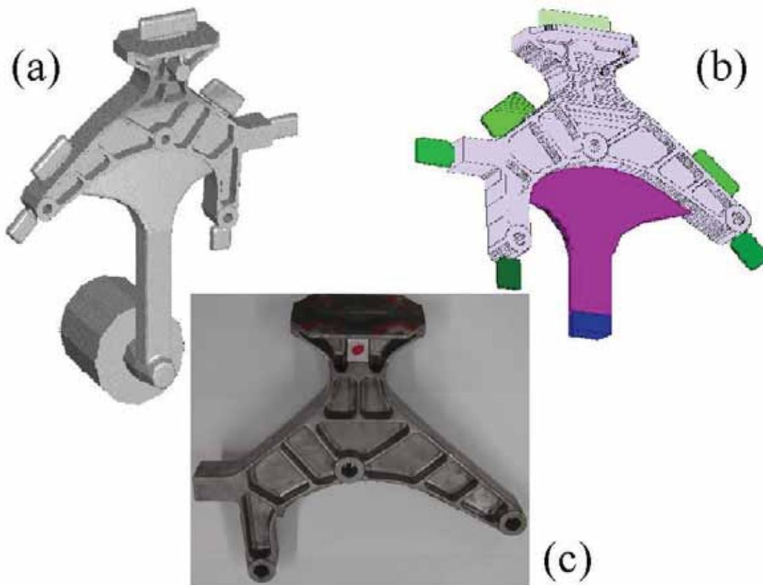
**Fig. 1:** 3D geometry of the engine bracket and of the casting system (a); 3D mesh developed for the numerical modelling (b); prototype of the engine bracket (c).
