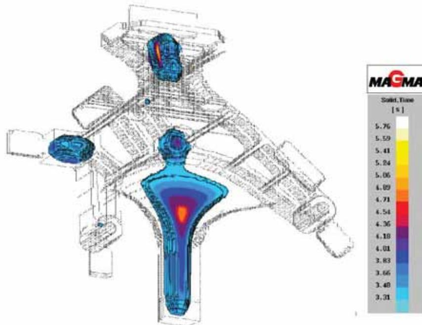
**Fig. 6:** Distribution of solidification times in the casting.
