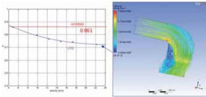
Fig. 4 - Loss coefficient curve for Bend Interaction.
