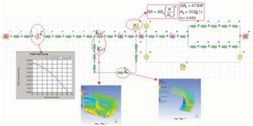
Fig. 8 - New System B Flowmaster model.
