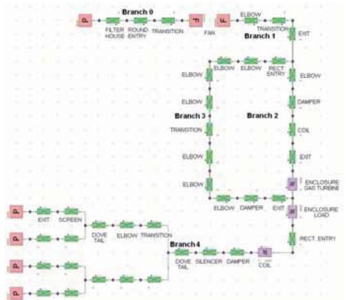
Fig. 1 - System A Flowmaster model based on discrete losses.
