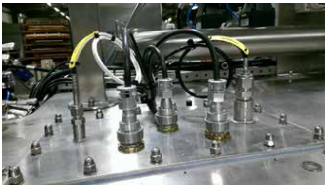
Fig. 6 - Anti-leakage bulkhead connectors
