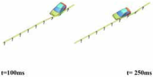
Figure 7. Performance of three shape rail
