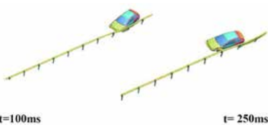
Figure 8. Performance of sigma shape rail
