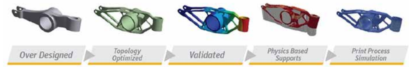
ANSYS simulation workflow for metal AM parts
