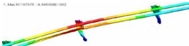
Figure 17. Deformation pattern for pipe diameter 90mm rail
