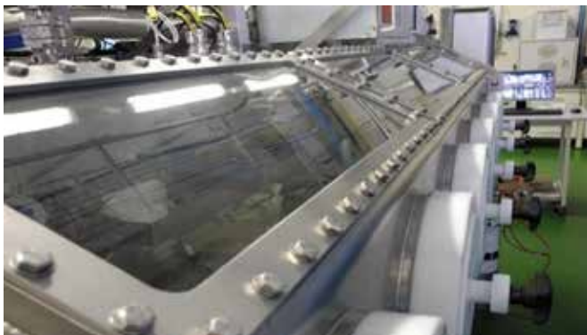
Fig. 7 - Anti-leakage fully bolted, gasketed joints
