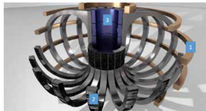
Magnet system: 1. Poloidal Field Coils - 2. Toroidal Field Coils - 3. Central Solenoid
