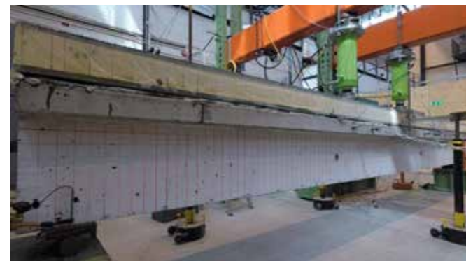
Figure 3 - Prototype beam strengthened with the SUREBridge technique and tested in the laboratory
