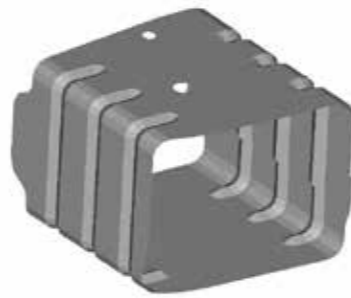
Figure 5 - First version of metallic Crash-Box
