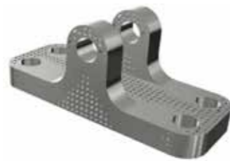
Structural lightening through a cellular microstructure in ANSYS SpaceClaim
