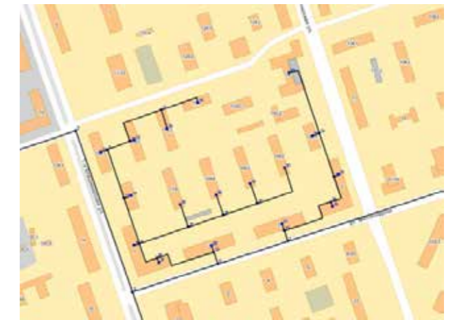
Fig.11 - District piping network on background map in Hydrosystem
