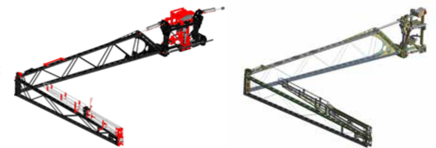
Figure 2 - On the left, original geometry for MY16 as received from CAD. On the right, geometry after the defeaturing process
