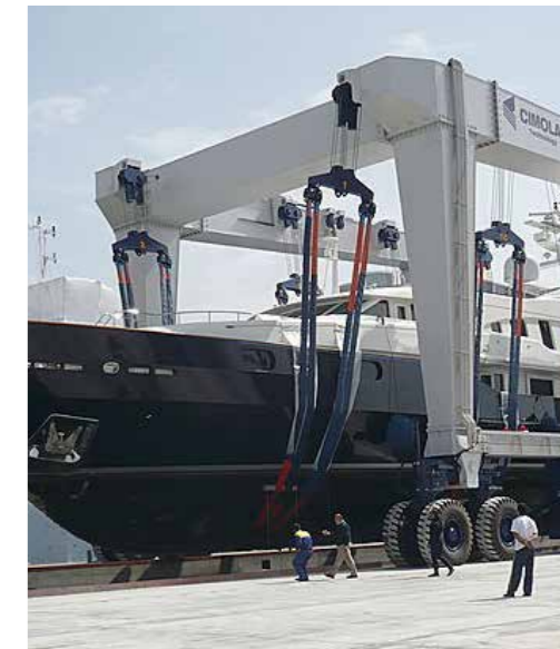
Fig. 2 - Mobile boat hauler for construction/repair yards
