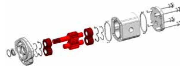
Figure 1b - POLARIS 20 pump exploded view
