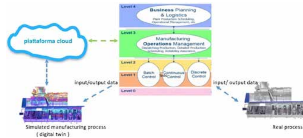
Fig. 2 -- ISA levels 95 and Digital Twin Project
