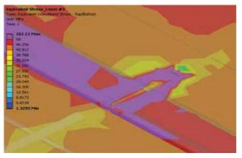
Figure 4 - von Mises stress induced by thermal cycling test
