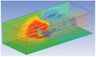
Figure 5 - Pressure Distribution and Velocity Streamlines
