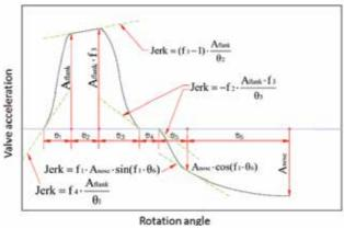
Figure 2 - Half-cam profile acceleration curve
