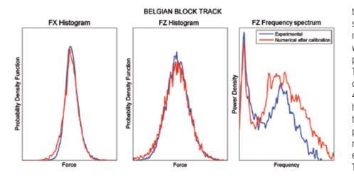
Figure 4 - Comparison between numerical and experimental histograms and spectra of the wheel forces measured on the Belgian block track
