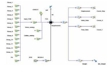
Figure 3 - Logic and data flow of the optimization process in modeFRONTIER
