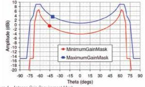
Figure 1 - Antenna Gain Requirement Mash
