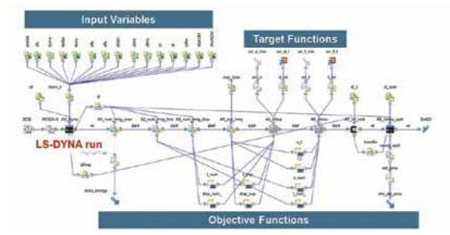
Figure 3- Sketch of the modeFRONTIER – LS-DYNA workflow
