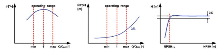
Figure 3 - left: Efficiency n; centre: suction capability NPSH within the operating range of the impeller dependent on the flow rate Q; right: NPSH3% criterion
