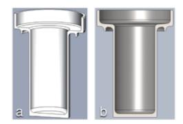
Figure 3 - a) Original geometry b) Manual optimized geometry
