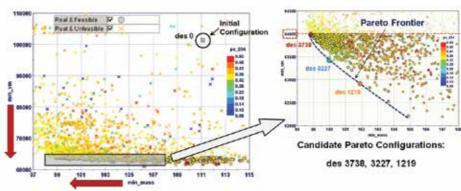
Figure 6 - Bubble Chart for multi-optimization - max of Von Mises stress vs. mass and Pareto Frontier
