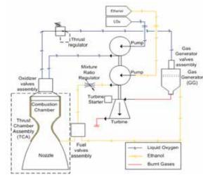
Figure 2 - L75 Engine cycle: gas generation
