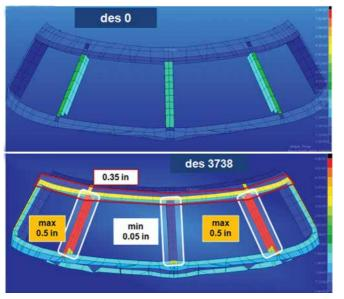
Figure 8 - FEM thicknesses – Comparison between baseline and optimum configurations
