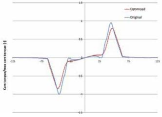
Figure 16 - Cam torque: comparison between original and optimized solution
