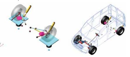
Figure 1 - Multibody Models: Rear Suspension and Full-Vehicle Handling Model - assembling Front Suspension, in a vehicle development project. Depending Steering system, Anti-roll-bar, Driveline, Engine, Rear Suspension, Body and Front & Rear Tires
