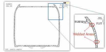
Figure 3 - Section of a carbody structure
