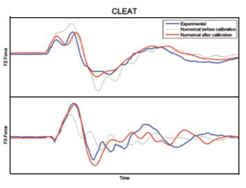
Figure 3 - Comparisons of experimental and numerical wheel forces on cleat and pothole
