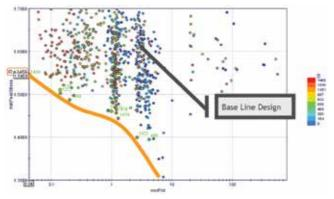
Figure 11 - The multi-objective optimization aims to reveal the Pareto front, marked by the orange line. The marked designs in the lower left corner represent the best trade-off designs between offset error and service life. Note the two zones with accumulation of designs which indicate some issue with the analysis
