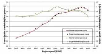
Figure 4 - Engine torque and power curves: comparison between measured and computed
