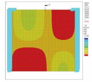
Figure 3.1.2 – Glass surface with the applied node-temperature
