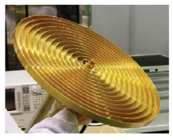
Figure 2 - Engineering Model of PDHT Isoflux Antenna with Several Series of Slots along Radial Direction
