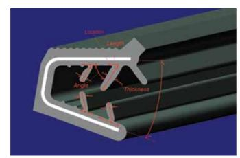
Figure 1 - Seal geometry
