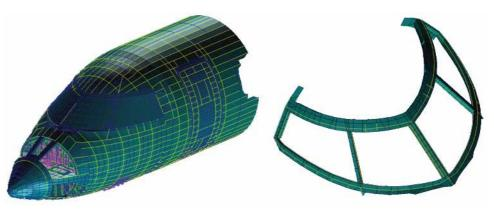
Figure 1 - GFEM: the finite element model of the Cockpit and the windshield alone
