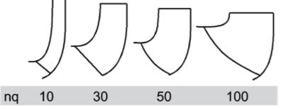
Figure 4 - Impeller form in meridional view dependent on specific speed n.
