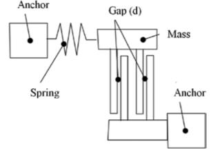
Figure 2 - A low-g accelerometer measures the change in capacitance with varying gap size. The gap, typically 1.5 to 3  $\mu$ m, changes when acceleration forces move the mass
