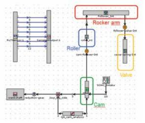
Figure 5 - Snapshot of the GT® valve train model
