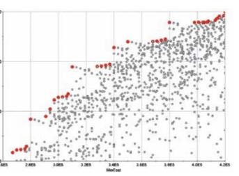
Figure 4 - Scatter plot representing the total cost and the minimum pressure level of each design; optimal designs are highlighted in red
