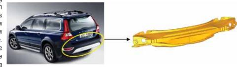
crash. Due to the complexity and cost of Figure 1 - Low speed crashes represent more than 70% of the crashes and combined with very high costs for repairs make robust design optimization extremely important. The study focuses on the bumper beam shown to the right
