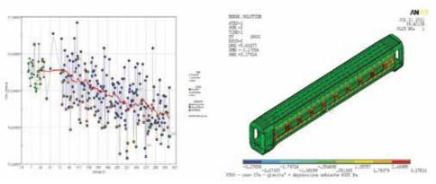
Figure 4a - History of weight convergence (green points: 1st optimization loop; blue points: 2nd optimization loop).
