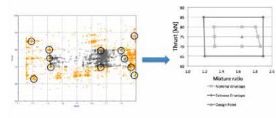
Figure 6 - TCA envelop operational space plot and optimal design
