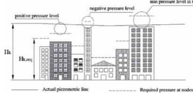
Figure 2 - Actual piezometric line (Hk) and required pressure at nodes (Hk,req) – from Nicolini (2005)
