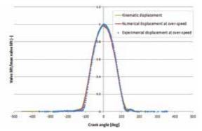
Figure 6 - Valve displacement: kinematic and dynamic profiles: comparison between measured and computed
