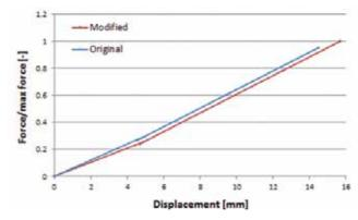
Figure 17 - Valve spring characteristics: comparison between original and modified solution
