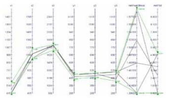
Figure 10 - The parallel coordinates chart shows both objectives and the input parameters in the same diagram for the 4 Pareto designs. Compared to the specified input ranges, showed by the full height of the axes, the Pareto designs are concentrated to a narrow zone. Based on this, the parameter ranges were reduced before starting the MOGA optimization
