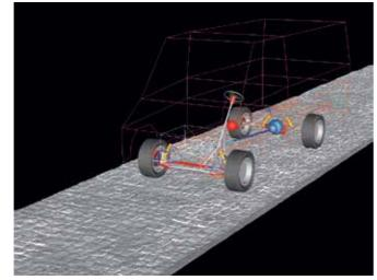
Figure 1 - Multi-body model of Iveco Daily driving on Belgian blocks test track
