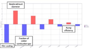
Figure 5 - Study on Specific Impulse main variables
