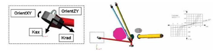
Figure 2 - Input variables: Rear suspension longitudinal arm attachment orientation and characteristics
