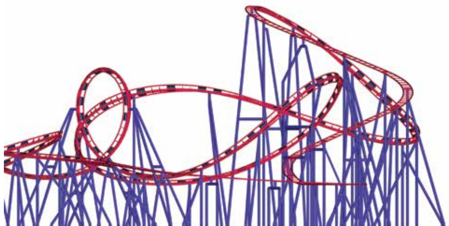
Fig. 1 - Loop 395 Coaster, side view of Finite Element Model
