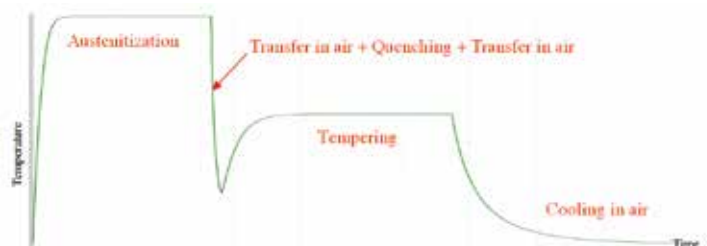
Fig. 1- wheel mean temperature during heat treatment
