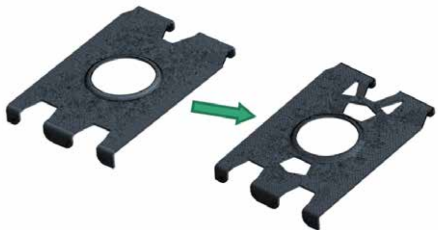
Fig. 5 – Lightening of the RTM carbon rib exploiting the results of the topological optimization
