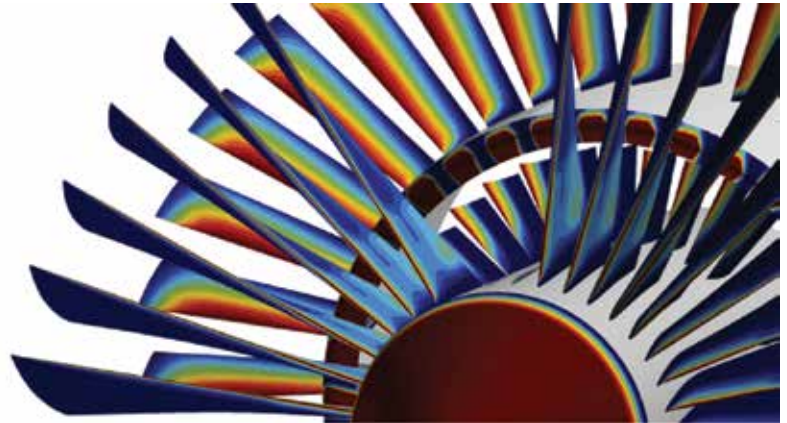
Fig. 4 - Ice Crystal impingement zones on engine surfaces
