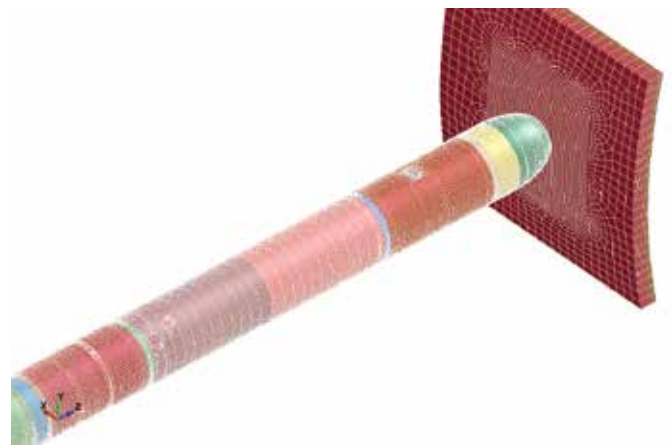
FE Torpedo impact on a target
