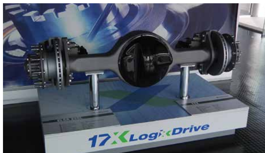
Figure 1 - The MS-17X single reduction hypoid drive axle
