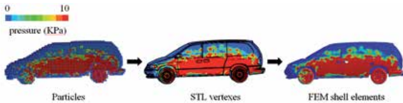
Fig.3 - Example of mapping results of pressure distribution at time = 0.85 sec.
