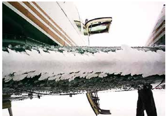
Figure 2 - Typical ice shape on the Leading Edge of a wing
