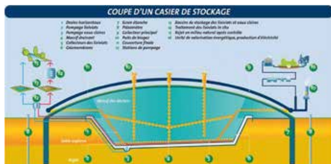
Fig. 1 – Principles and cross-section of a storage compartment
