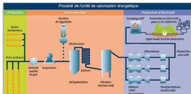
Fig. 2 – Biogas valorization principles
