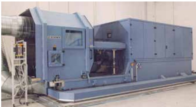
Fig. 1 - POLI SpA test bench can simulate any braking condition up to a speed of 450km/h
