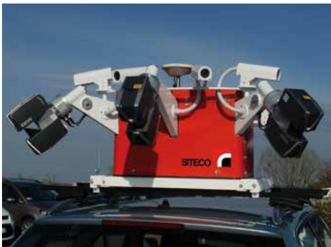
Fig. 1 - The Road-Scanner3 Mobile Mapping System
