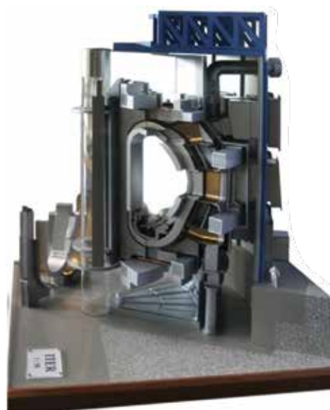
Fig. 1 - Cross section of ITER. It should be noted the dimension of the white dressed technician placed on the right with regard to ITER reactor
