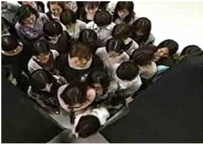
Prof. Nishinari's experiment to look at the effect of a column in front of the exit
