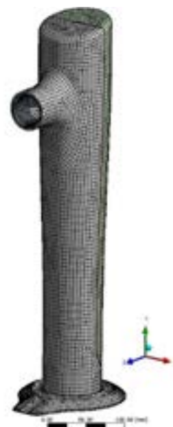
Fig. 2 - FE model of the fount
