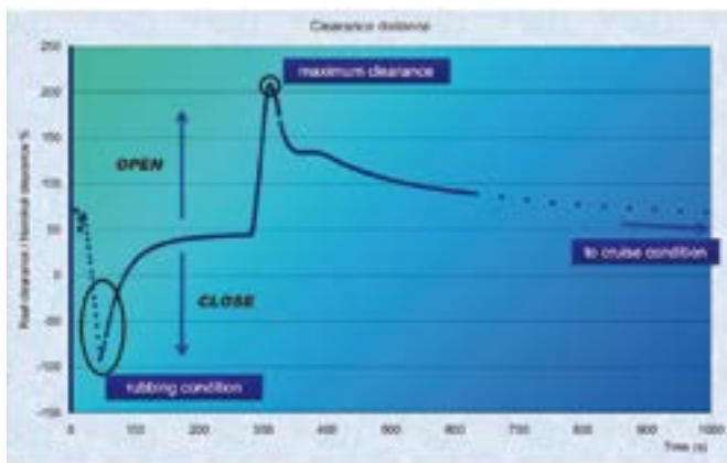
Fig. 4 - Results of an integrated multi-physics simulation of the entire engine mission: clearance (%)
