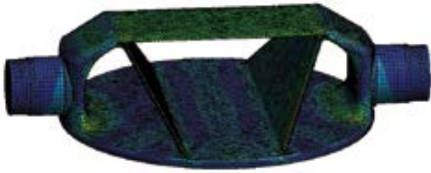
Von Mises stress distribution at Valve Disc for Valve in closed condition
