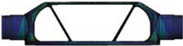
Von Mises stress distribution at Valve Disc for Valve in closed condition
