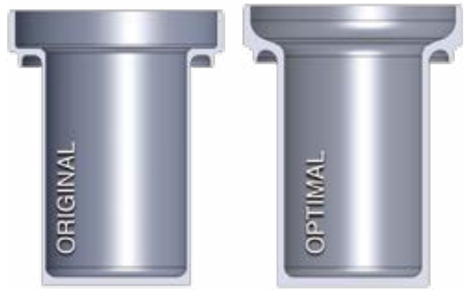
Fig. 9 - Original 16 mm piston (LEFT) and Optimal piston as result of automatic optimization process
