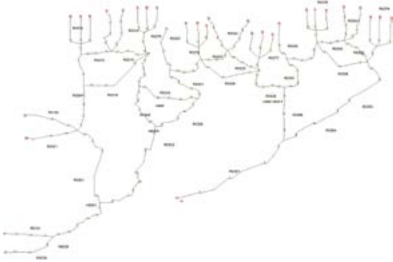
Fig. 3 - Example of a Flowmaster network for the system level fluid-dynamic simulations
