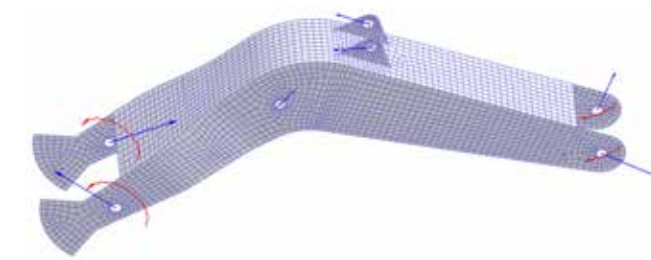
Figure 3 – FE analysis of the excavator boom. The FE model is loaded with forces and torques calculated through rigid MBS
