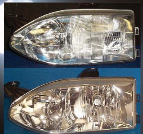
Figure 1: Comparison Between an Old Fashioned Glass Headlamp (top) and a New Transparent Plastic Headlamp (bottom)
